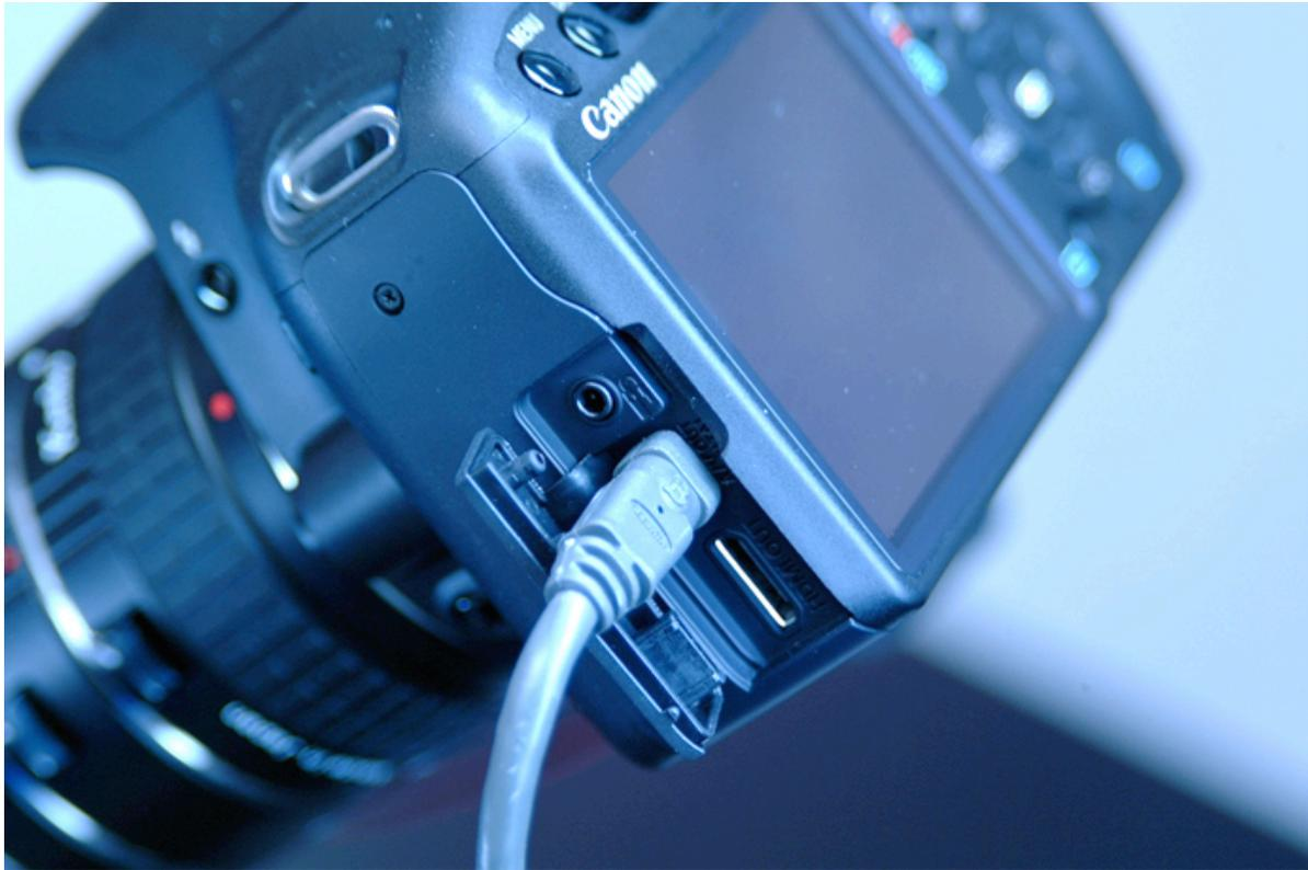
The power supply should be connected to to an appropriate surge protected 110-volt or 220-volt power source on one end and to the SpotBot® 3 Advanced Vision System camera as shown here. The power supply allows continuous use of the digital camera without depleting the camera's batteries.
